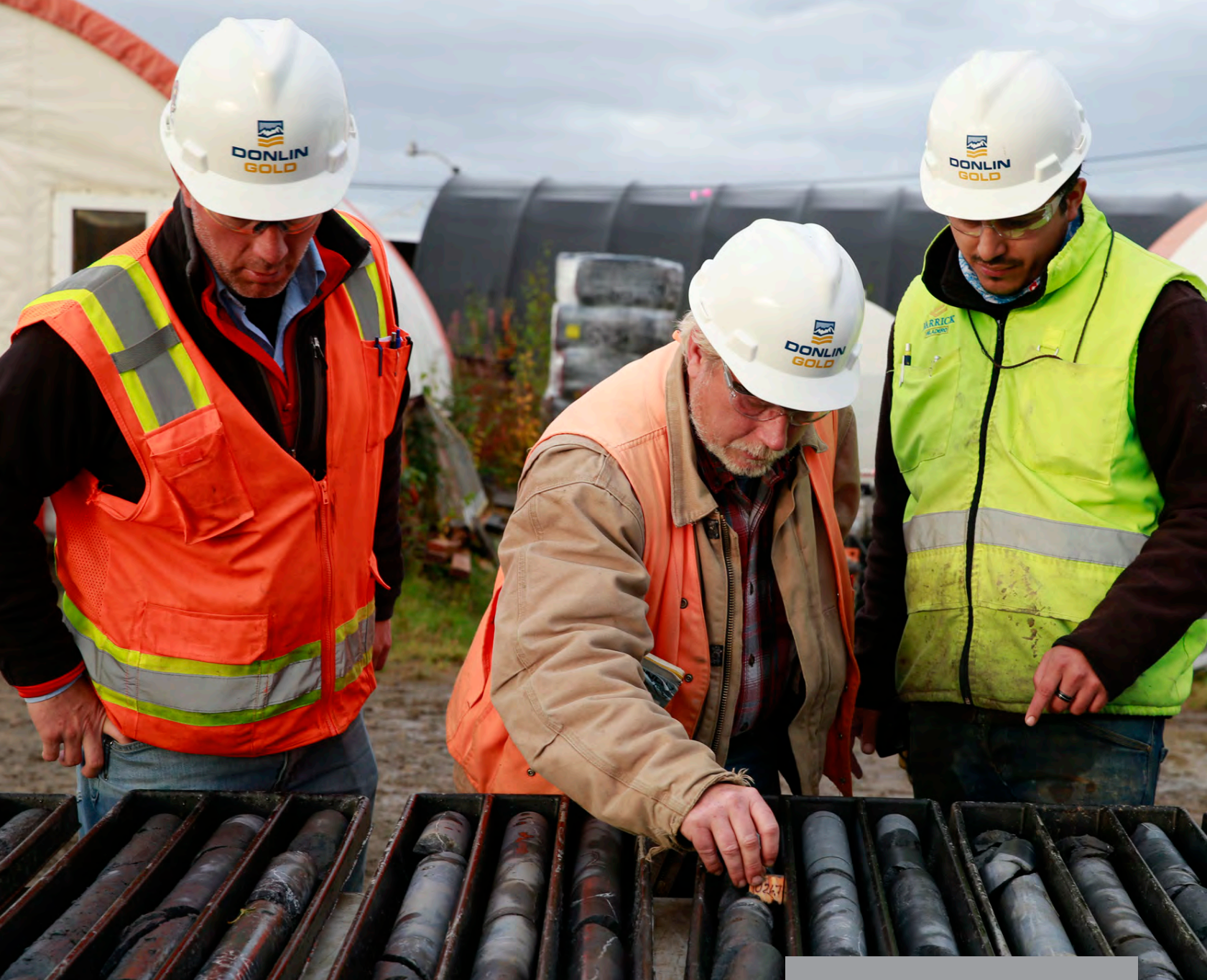
Drill core is logged onsite before being transported to assay labs for evaluation.
